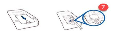
(7) – Connect your network/internet cable to the (ETH) port, and the power cord to the card terminal dongle.
